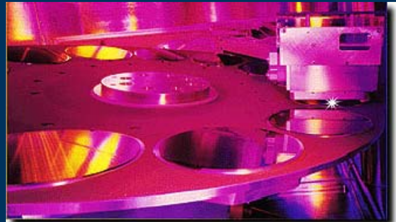
Ion Implanter Wafer Handling Mechanism (Varian Associates)
